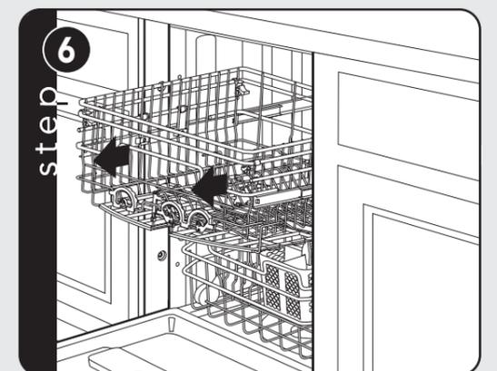
To check level, front to back, pull the top rack half-way out of unit. The rack should remain stationary and not move in or out.
