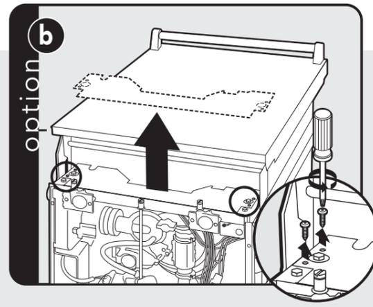
Remove bottom pan and front plate.
