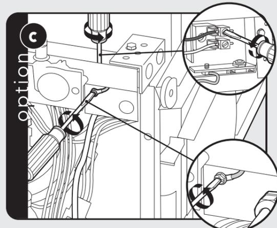
Loosen ground wire and wires on terminal block. Loosen strain relief and remove cord. **NOTE:** Other items are grounded in this location—these items must remain grounded.
