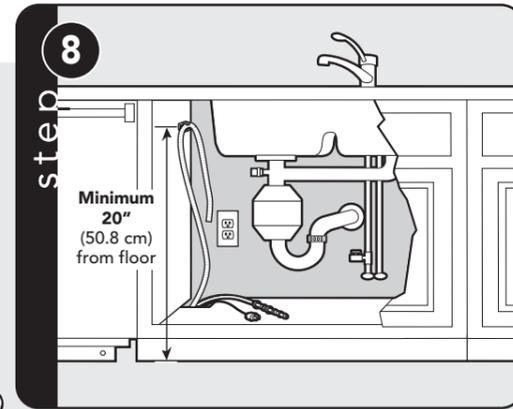
Install High Loop Clip, which is provided, a minimum of 20" (50.8 cm) from the floor.
