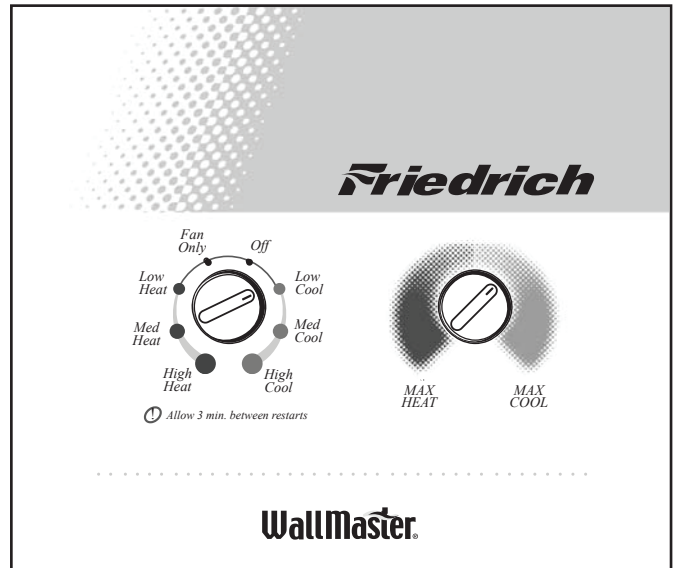
Figure 7: System Control Panel
