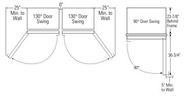
Allow 25" minimum clearances for a full 130° door swing. Allow 15" for pan removal.
