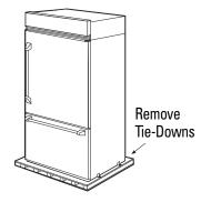
• Remove the four 7/16" bolts securing the straps to the skid.
