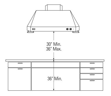
\*9" for ceiling heights of 7' 11" to 8' 5" using the supplied support frame and duct cover.
