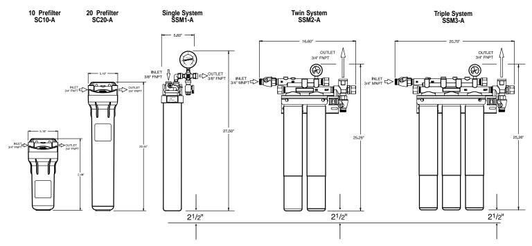
IMPORTANT: Must have minimum 21/2" clearance for cartridge change.
