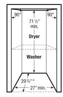
Stacked Units in Recessed or Closet Installation For detailed stacked installation, refer to instructions included with Stacking Kit or on web. Note: Stacked installation requires modified utility hookup locations
