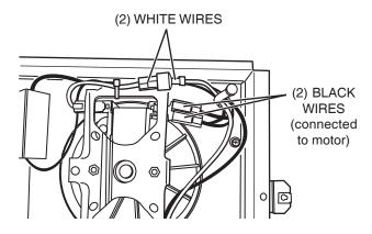
2)Connect the two (2) white wires with insulated terminals to each other.
