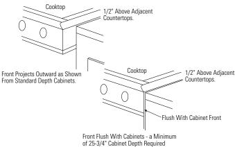
NOTE: These cooktops require 8" free space below the countertop to house the cooktop burner box. Allow additional clearances below the burner box to install the regulator and make house gas supply connections. Use a 90° elbow to route the gas connections and limit interference with drawers or other cabinetry features.
