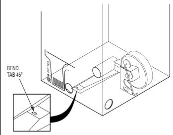
Through the rear opening, locate the tab in the middle of the appliance base. Lift the tab to about  $45^{\circ}$  using a flat blade screwdriver.
