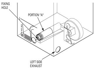
Reconnect the cut portion (A) of the duct to the blower housing. Make sure that the fixing hole is aligned with the tab in the base. Use the screw saved previously to secure the duct in place through the tab on the appliance base.
