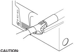
Internal duct joints must be secured with tape, otherwise they may separate and cause a safety hazard.
