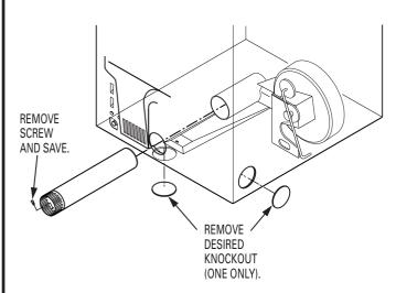
Detach and remove the bottom or left side knockout as desired. Remove the screw inside the dryer exhaust duct and save. Pull the duct out of the dryer. Protect sharp edges around the knockout and exhaust opening with tape.
