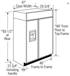
\* Shipping height. The refrigerator can be adjusted to fit into a cutout that is 83-1/2" min. to \*84" From 84-1/2" max. height. Floor to Top Frame case trim at the front is 1/2" higher and will overlap upper cabinetry or soffit. Use leveling legs and wheels for a maximum 1" height adjustment.
