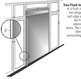
**True Flush Installation** In a flush installation. the refrigerator door will align evenly with the front face of adjacent cabinet doors. The refrigerator blends into the surrounding cabinetry.
