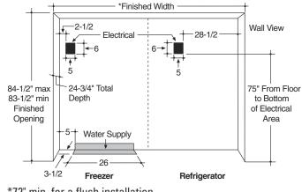
\*72" min. for a flush installation 71-1/2" min. for a semi-flush installation
