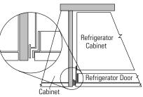
Note: 1/2" thick side panels shown. Side panels can be any thickness. Add side panel thickness to outside trim width (36" or 72" for two models) to calculate the rough-in dimension. The leading (front) edge must be finished to match surrounding cabinetry.
