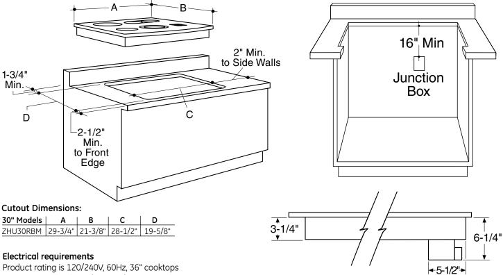
Product rating is 120/240V, 60Hz, 36" cooktops to a 50-amp circuit; and 30" cooktops to a 40-amp circuit. The cooktops must be connected to a supply circuit of the proper voltage and frequency and protected by a time-delay fuse or circuit breaker.
