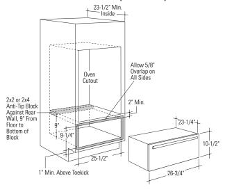
**Note:** Additional clearance between cutouts may be required. Check to be sure that oven supports above the Warming Drawer location do not obstruct the required interior 23-1/2" depth and 9-1/4" height.
