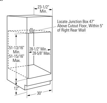
The solid bottom or runners must be level with the bottom of the cutout, or the bottom trim may not install correctly and could interfere with the door opening. If the cabinet does not have a solid bottom, two braces or runners must be installed level with the bottom of the cutout to support the weight of the oven. The runners and braces must support 375lbs. (90 kg).
