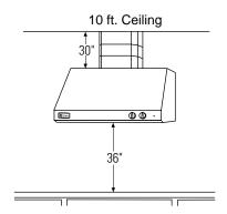
10 ft. ceilings: When the hood is installed 36" above the cooking surface, order three 12" and
