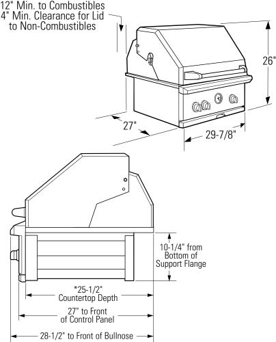
\*The weight of the grill is fully supported by the side trims. The back of the grill overlaps the back edge of the cutout.
