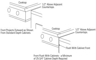
NOTE: These cooktops require 8" free space below the countertop to house the cooktop burner box. Allow additional clearances below the burner box to install the regulator and make house gas supply connections. Use a 90° elbow to route the gas connections and limit interference with drawers or other cabinetry features.
