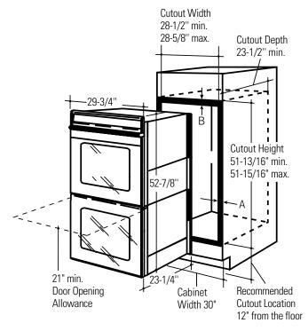
**Note:** Most 30" wall cabinets can be used with this unit. The opening between the inside walls must be at least 28-1/2" wide.
