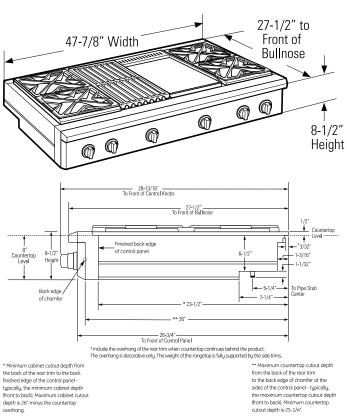
Allow 8" free space below the top surface of countertop. Allow additional clearances below the burner box to install the regulator and make house gas supply connections. Use a 90° elbow to route the gas connections and limit interference with drawers or other cabinetry.
