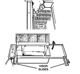
Pull the visor slides out. Rotate the panel clips and swing the panel open.
