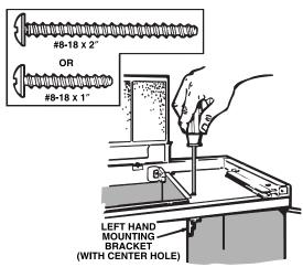
Two (2) sets of screws are provided. Use the short screws for flush bottom cabinets or long screws for recessed bottom cabinets. Insert two (2) screws through the housing and into the mounting bracket. Do not tighten screws completely.
