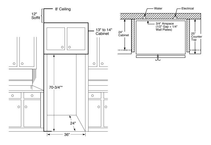
\*The rough-in dimension of 70-3/4" is minimum and is measured from the finished floor to top of opening (or the underside of the overhead cabinets). For Models with Trim Kit: If frameless style cabinets are planned for above the refrigerator, you may need to consider adding a maximum of 1/4" (71") to height of opening to allow additional clearance between cabinet doors and top of refrigerator trim when cabinet doors are in open position.
