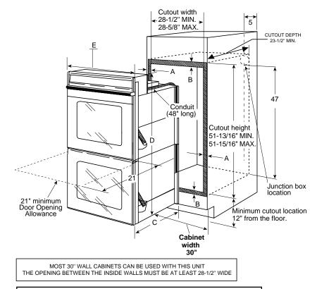
Electric wall ovens are not approved for installation with a plug and receptacle. They must be hard wired in accordance with installation instructions.
