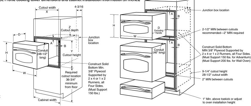
A=Allow 1" overlap of oven over top and bottom edges of cutout. B=Allow 11/16"-3/4" for overlap of oven over side edges of cutout. A=Allow 1" overlap of oven over top and bottom edges of cutout. B=Allow 11/16"-3/4" for overlap of oven over side edges of cutout.
