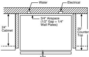
\*The rough-in dimension of 70-1/4" is minimum and is measured from the finished floor to top of opening (or the underside of the overhead cabinets). For Models with Trim Kit: If frameless style cabinets are planned for above the refrigerator, you may need to consider adding a maximum of 1/4" (70-1/2") to height of opening to allow additional clearance between cabinet doors and top of refrigerator trim when cabinet doors are in open position.
