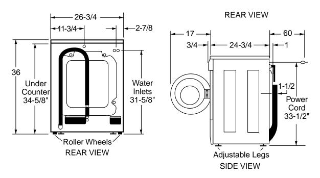
**Electrical Requirement:** 120Volts, 60 Hertz. An individual, properly grounded 20-amp branch circuit is required.
