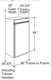
\*Shipped at 84" installation height. Can be adjusted to 83-1/2" or 84-1/2" with Grille Panel Kits.
