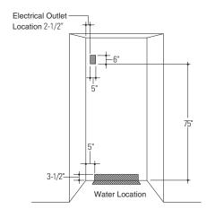
**Important**: To insure a flush fit and access to the power cord, locate the electrical outlet as shown.
