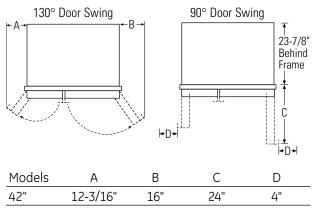
Allow minimum clearances for Freezer door (Dimension A) and Fresh Food door (Dimension B) for a full 130° door swing and to allow for drawer removal.
