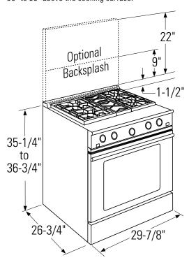
Clearances between range and side wall or combustible material must be at least 12" on each side.
