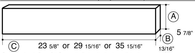
\* If you wish to keep the frame of the front panel and only replace the glass panel, the dimensions are as follows:
