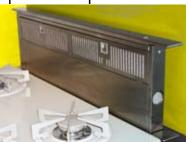
Rising a full 8 1/4" above the cooktop, the Scirocco vents horizontally across the cooking surface and down through the exhaust vent. At the press of a button, the stainless steel Scirocco retracts back down into the counter. Momentary delay up/down
