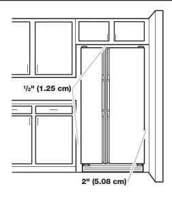
To ensure proper ventilation for your refrigerator, allow for  $\frac{1}{2}$ " (1.25 cm) space on each side and at the top. When installing your refrigerator next to a fixed wall, leave 2" (5.08 cm) minimum on each side (depending on your model) to allow for the door to swing open. If your refrigerator has a water dispenser and ice maker, allow extra space at the back for the water line connections.
