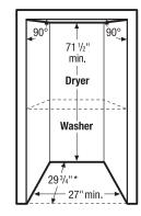
Stacked Units in Recessed or Closet Installation For detailed stacked installation, refer to instructions included with Stacking Kit or on web. **Note:** Stacked installation requires modified utility hookup locations for dryer. For details, refer to Product Installation Guide on web.
