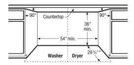
Side-by-Side Units in Under-Counter Installation Can be installed with standard countertop and/or cabinetry.
