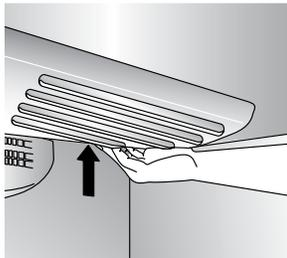
3. If your refrigerator has a dispenser system with water filter, remove the water filter cartridge and install the filter bypass. Dispose of the used cartridge.
