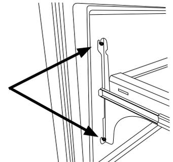
4. Lift the drawer front upward and off the screws.
