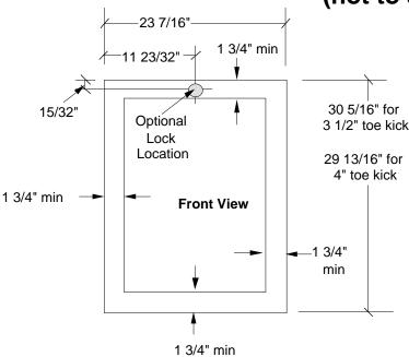
For doors with locks installed (-LR or -LL included in model number). It will be necessary to drill a hole in the overlay door frame, corresponding to the lock location, prior to assembly. Hole diameter through overlay frame should be 15/32" with a 13/16" counterbore from back side of panel, 7/16" deep.
