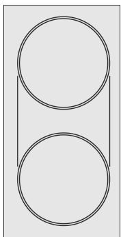
The Bridge element combines two individual heating elements into one long griddle zone. This configuration is ideal for griddles and large pans.
