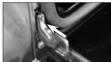
Fig. 08 Hinge retainer clip in locked position
