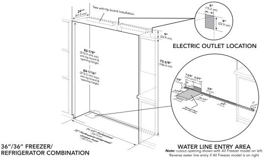
\*Custom front models fit flush in 25"-deep (63.5 cm) cabinet openings. They can be installed in standard 24"-deep openings. The door faces and top grille will protrude 3/4" (1.9 cm) into the room.
