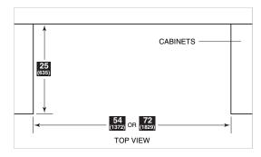
Installation of two units side by side
