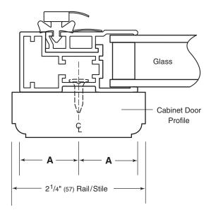
This full-scale illustration is typical of the Model 424 door frame profile; details of the other Wine Storage door frames will vary slightly.
