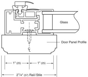
The full-scale illustration shows the door frame profile for Model UC-24B.
