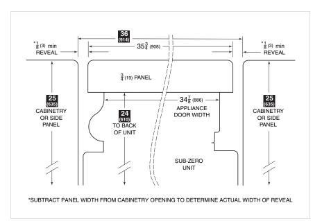
Dimensions are in inches with millimeters in parentheses unless otherwise specified.
