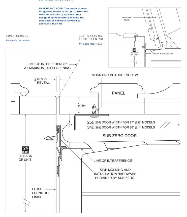
\*If the panel is thicker than 3/4" (19), it is recommended that you utilize the built-in 90° door stop to prevent damage to the panel and face frame.
