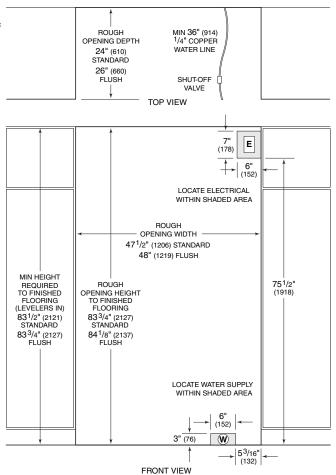
Refer to the fullscale illustrations at the end of this section for specifics on door openings and other specifications.
