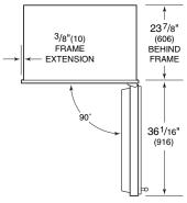
SHUT-OFF VALVE TOP VIEW 351/2" (902) ROUGH OPENING WIDTH 72<sup>3</sup>/4" (1848) ROUGH OPENING 72<sup>3</sup>/4" (1848) MINIMUM HEIGHT **HEIGHT TO** REQUIRED TO FINISHED FLOORING (LEVELERS IN) FINISHED FLOORING LOCATE ELECTRICAL WITHIN ENTIRE SHADED AREA LOCATE WATER SUPPLY WITHIN BOTTOM SHADED AREA ONLY (601F ONLY) 6" (152) 24" (610) 3" (76) Е 11' (W) FRONT VIEW
