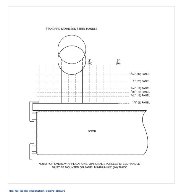
handle placement for the standard stainless steel handle on the wrapped stainless steel door and on overlay panel applications shown in the dashed line.
