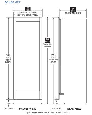
Dimensions in parentheses are in millimeters unless otherwise specified. INTEGRATED PANEL SPECIFICATIONS
