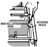
Insert the bent end of the installation rod into the access hole in the housing.
