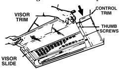
Slide the glass into the visor slides, above each visor clamp (see the illustration in step 14). Align the visor trim and tighten the thumb screws to secure the glass.
