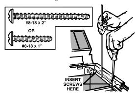
Hold the mounting bracket in place with the rod. Two sets of screws are provided. Use the short screws for flush bottom cabinets or the long screws for recessed bottom cabinets. Insert two (2) screws through the housing and into the mounting bracket. Do not tighten the screws completely.
