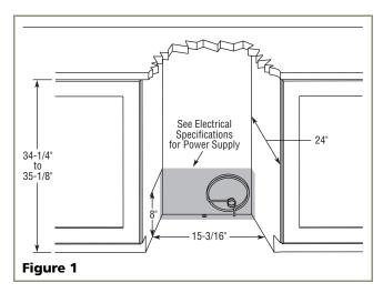
Follow the cut-out drawing in **Figure 1**. The 15-3/16" width allows 1/4" for ease in installation and removal of the unit. 24" is the cabinet depth in most installations. The unit is 23-11/16" deep including the handle on Black and White models and 23-11/16" deep including the door and *not* the handle on Stainless Steel models (see **Figure 2**).
