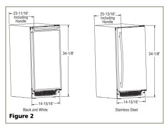
Please note that the unit has adjustable feet that can add one additional inch to height during leveling or to match adjacent cabinets (see **Figure 36** on **Page 14**).
