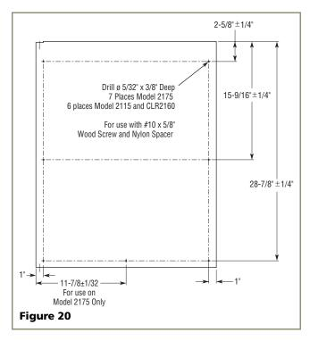
3. Attach the door panel to the overlay panel using #10 x 5/8" wood screws and nylon spacers. The nylon spacers fit between the overlay panel and the door panel as shown in **Figure 21**. The spacers allow the original door panel to slide back into the 1/4"-thick door reveal (channel).
