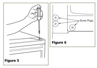
3. Remove top hinge (3 screws), reinstall hinge screw pin, and remount on opposite side BOTTOM (see **Figure 7**).
