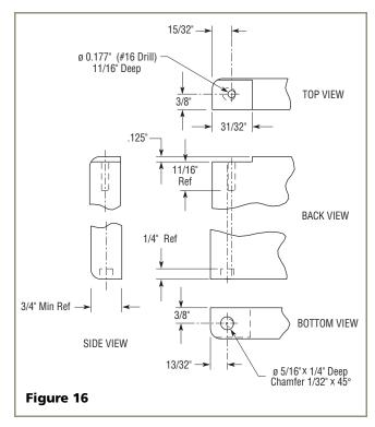
Route notch in top corner of overlay panel as shown (see Top and Side Views). Top of notch is entire depth of panel, front to back.
