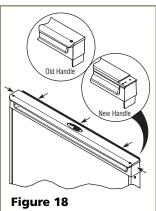
Remove the two screws located on both sides of the handle.
