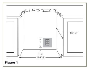
Follow the cut-out drawing in **Figure 1**. The 24-3/16" width allows 1/4" for ease in installation and removal of the unit. 24" is the cabinet depth in most installations. The unit is 23-1/4" deep including the wood overlay frame on 2175BEVOL2 models and 23-1/4" deep including the door and *not* the handle on Stainless Steel models (see **Figure 2**).
