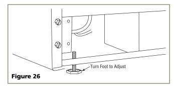
3. Check the levelness after each adjustment and repeat the previous steps until the unit is level. Go on to **8 Install the Unit**.
