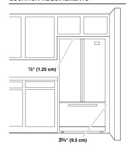
To ensure proper ventilation for your refrigerator, allow for a ½" (1.25 cm) space at the top and behind the refrigerator. If your refrigerator has an ice maker, allow extra space at the back for the water line connections. When installing your refrigerator next to a fixed wall, leave 3¾" (9.5 cm) minimum space between the refrigerator and wall to allow the door to swing open.
