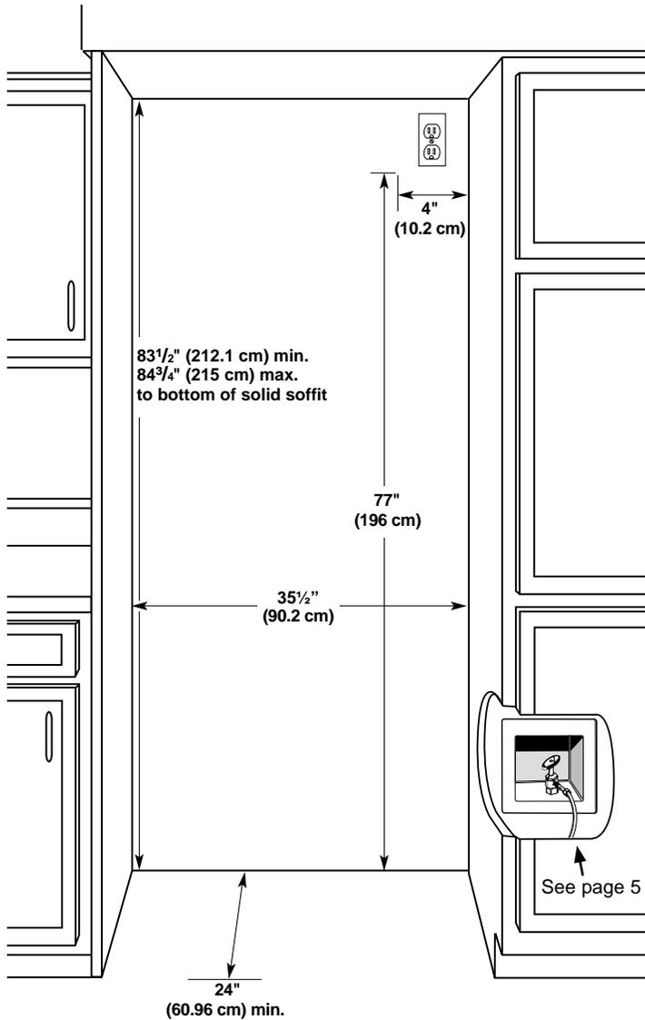
**NOTE:** Flooring under refrigerator must be at same level as the room. Face of cabinet must be plumb.
