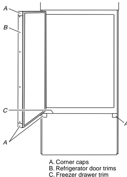
4. Slide the custom panels into the bottom and hinge side trims on the refrigerator compartment and freezer compartment doors, making sure that the backer panel fits into the hinge side trims.
