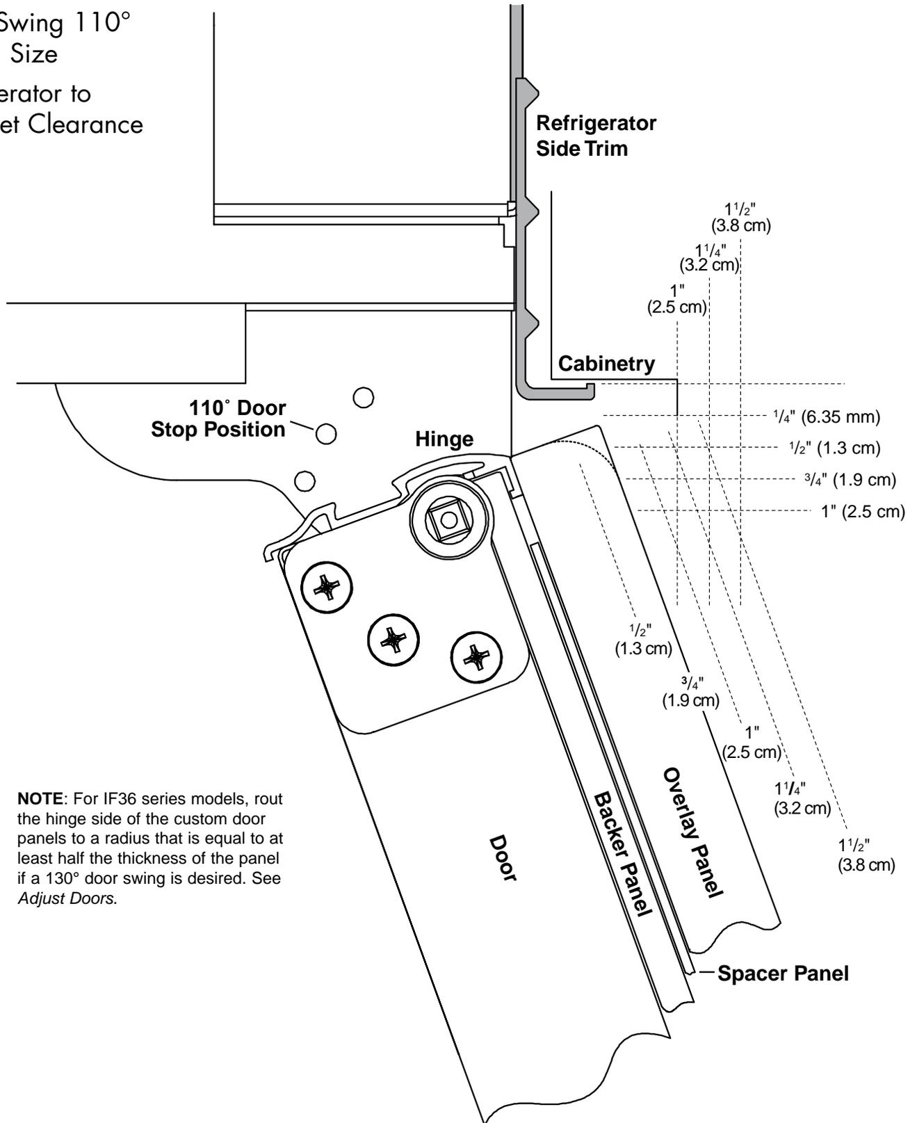
**NOTE:** For IF36 series models, rout the hinge side of the custom door panels to a radius that is equal to at least half the thickness of the panel if a 130° door swing is desired. See *Adjust Doors*.
