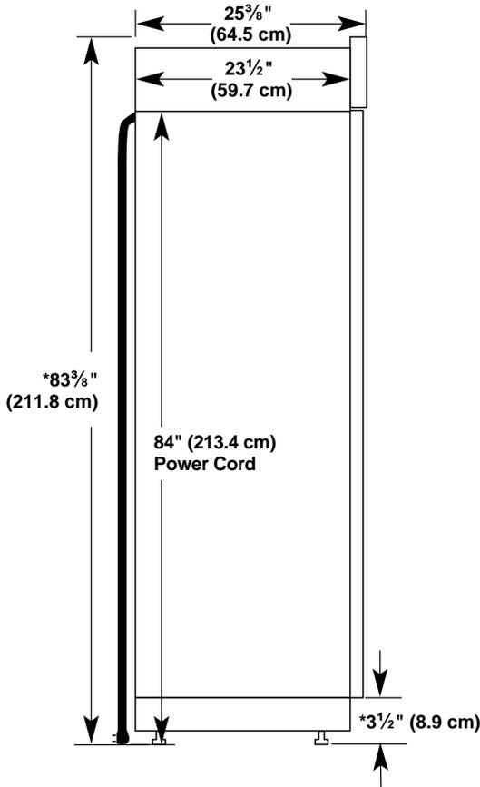
\* When leveling legs are fully extended to 1<sup>1</sup>/<sub>4</sub>" (3.2 cm) below rollers, add 1<sup>1</sup>/<sub>8</sub>" (2.9 cm) to the height dimensions.
