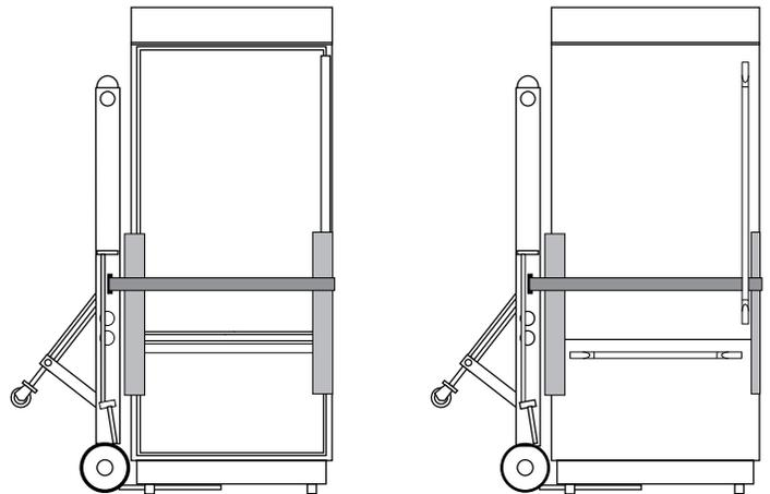
2. Place pieces of the shipping carton on the floor when rolling the dolly and refrigerator into the house. Move the refrigerator close to the built-in opening.
