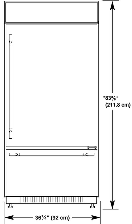
\* When leveling legs are fully extended to 1<sup>1</sup>/<sub>4</sub>" (3.2 cm) below rollers, add 1<sup>1</sup>/<sub>8</sub>" (2.9 cm) to the height dimensions.
