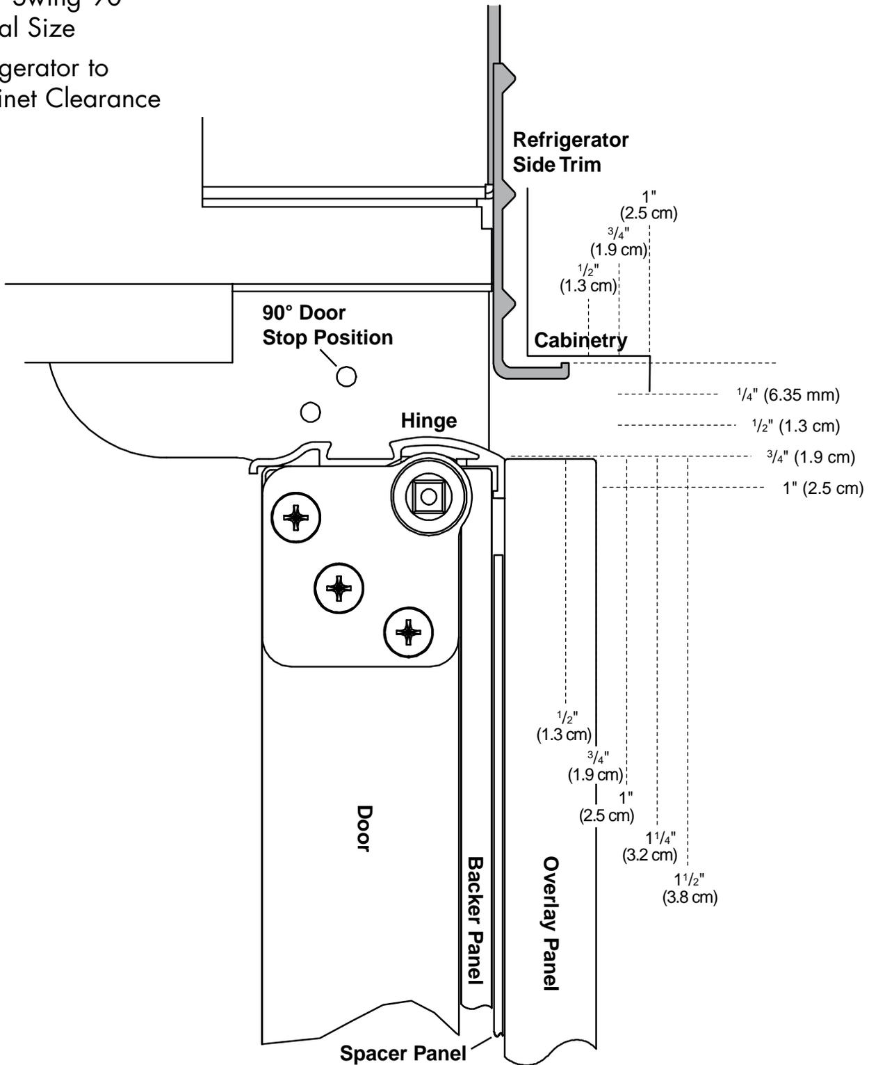
Allow a minimum of 4 1/2" (11.4 cm) of space between the side of the refrigerator and a corner wall. More clearance may be needed if thicker custom panels or custom handles are used. Do not overlook baseboards.
