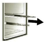
While supporting door front, hook supports into slots located on inside of each slide.
