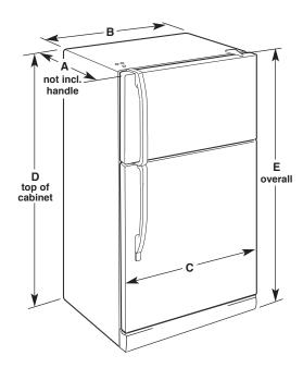
Dimensions "D" and "E" include rollers extended 3/4".
