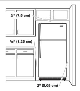
To ensure proper ventilation for your refrigerator, allow for a 1/2" (1.25 cm) space on each side and at the top. When installing your refrigerator next to a fixed wall, leave 2" (5.08 cm) minimum on the hinge side (some models require more) to allow for the door to swing open. If your refrigerator has an ice maker, allow extra space at the back for the water line connections.
