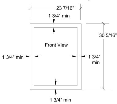
Min. thickness of rails and stiles: 5/8" Max. thickness of rails and stiles: 3/4"
