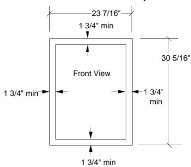
Min. thickness of rails and stiles: 5/8" Max. thickness of rails and stiles: 3/4"
