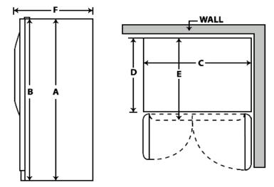
Allow 2" of clearance on hinge side of refrigerator when installing next to a wall where handle may make contact.
