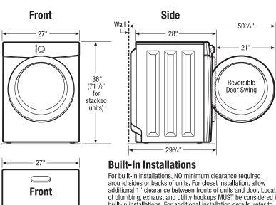
additional 1" clearance between fronts of units and door, Location of plumbing, exhaust and utility hookups MUST be considered in built-in installations. For additional installation details, refer to Product Installation Guides on web
